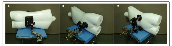
Fig. 1 Pelvic positioner (a) left, posterior support over the sacrum; (b) middle, anterior single support over the pubic symphysis (pubic support type); and (c) right, anterior double supports over the bilateral anterior superior iliac spine (ASIS type)
