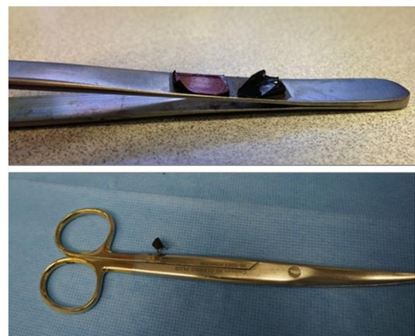
**Figure 2** Defective Labels: Top panel - Delaminating tape label peeling off a surgical forceps; Bottom panel - Fragmented plastic coating which broke off the end of a scissor during a surgical case.
