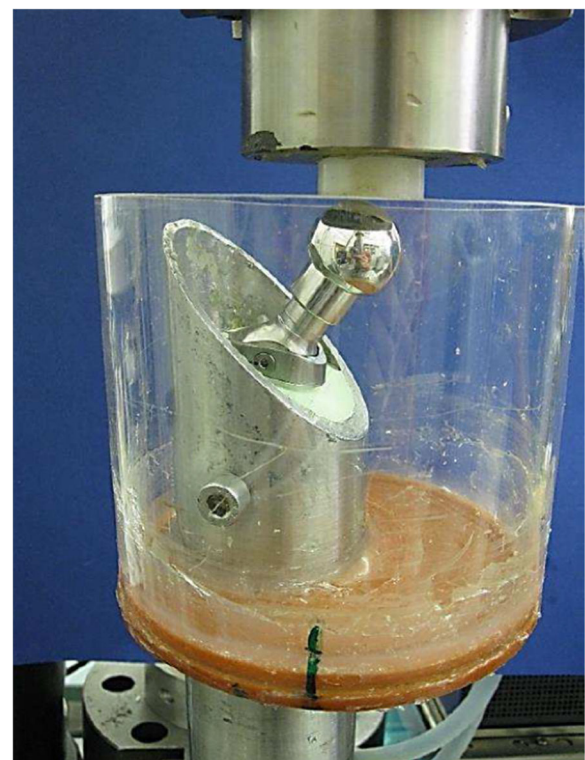
Fig. 3 Experimental setup for dynamic fatigue limit testing according to the ISO 7206–6 standard
